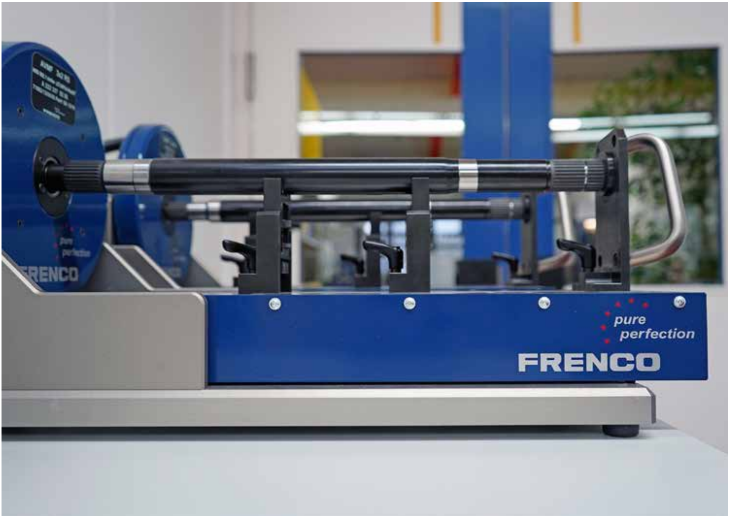
A close-up of the Frenco external gear and spline inspection instrument. (Courtesy: Euro-Tech)
